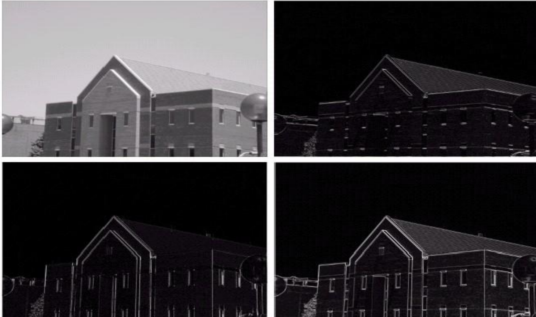
FIGURE 10.11 Same sequence as in Fig. 10.10, but with the original image smoothed with a 5 \times 5 averaging filter.
