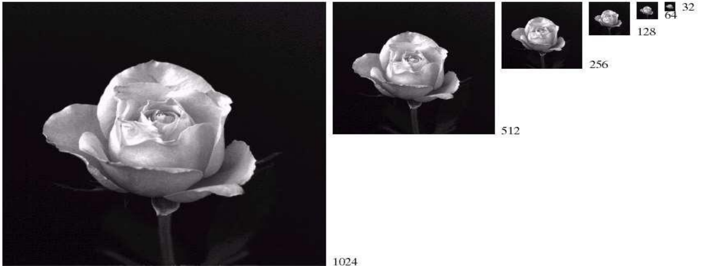
FIGURE 2.19 A 1024 \times 1024 , 8-bit image subsampled down to size 32 \times 32 pixels. The number of allowable gray levels was kept at 256.
