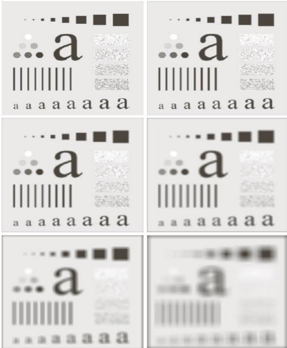
FIGURE 3.33 (a) Original image, of size 500 \times 500 pixels. (b)–(f) Results of smoothing with square averaging filter masks of sizes m = 3, 5, 9, 15, and 35, respectively. The black squares at the top are of sizes 3, 5, 9, 15, 25, 35, 45, and 55 pixels, respectively; their borders are 25 pixels apart. The letters at the bottom range in size from 10 to 24 points, in increments of 2 points; the large letter at the top is 60 points. The vertical bars are 5 pixels wide and 100 pixels high; their separation is 20 pixels. The diameter of the circles is 25 pixels, and their borders are 15 pixels apart; their intensity levels range from 0\% to 100\% black in increments of 20\% . The background of the image is 10\% black. The noisy rectangles are of size 50 \times 120 pixels.
