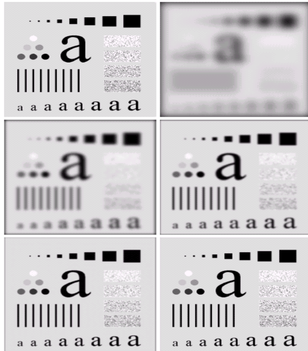
FIGURE 4.18 (a) Original image. (b)–(f) Results of filtering with Gaussian lowpass filters with cutoff frequencies set at radii values of 5, 15, 30, 80, and 230, as shown in Fig. 4.11(b). Compare with Figs. 4.12 and 4.15.
