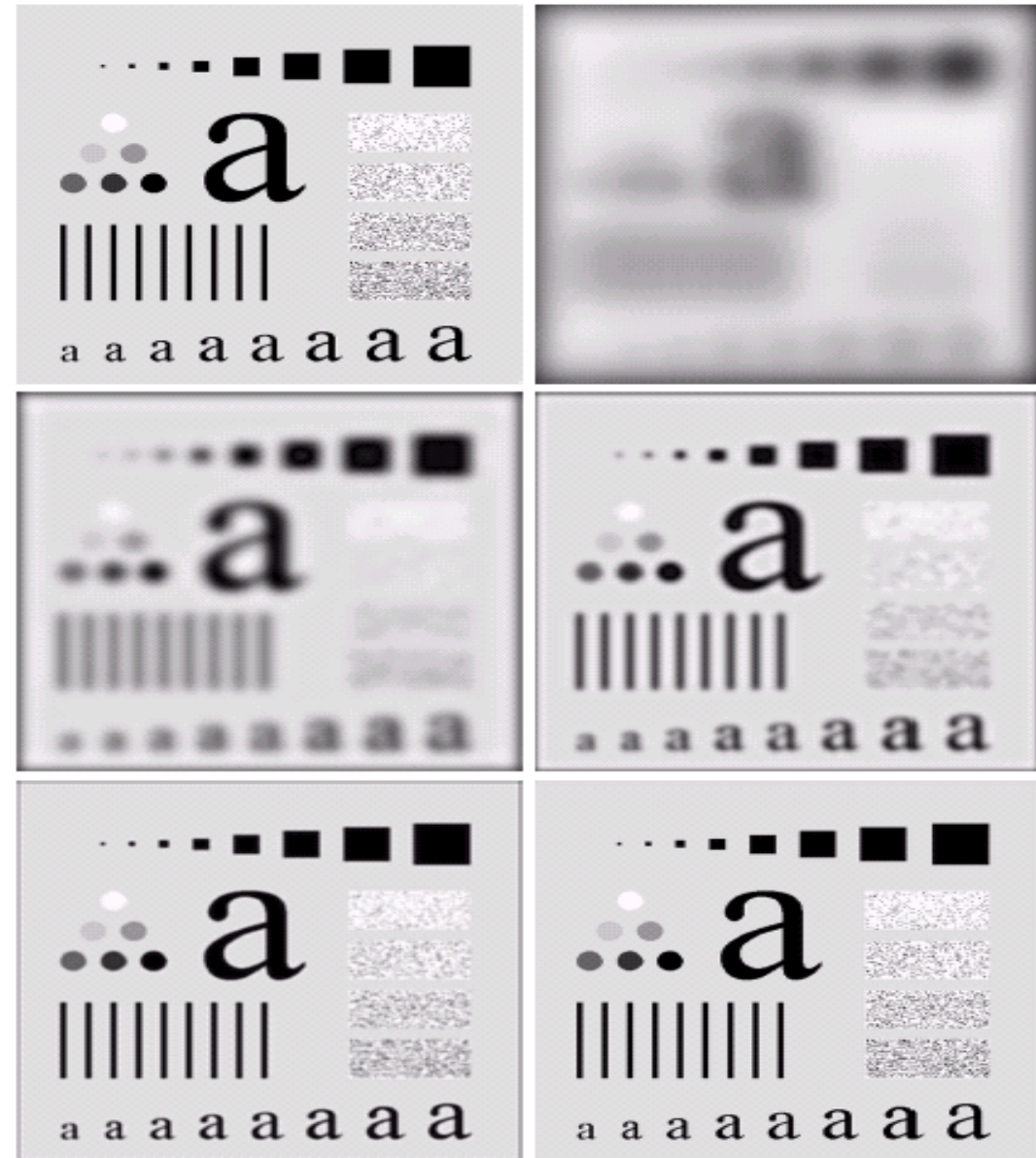
FIGURE 4.15 (a) Original image. (b)–(f) Results of filtering with BLPFs of order 2, with cutoff frequencies at radii of 5, 15, 30, 80, and 230, as shown in Fig. 4.11(b). Compare with Fig. 4.12.
