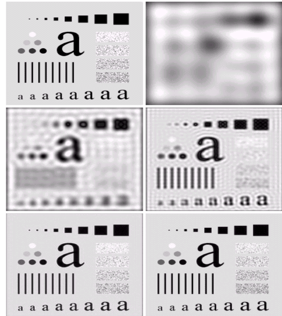
FIGURE 4.12 (a) Original image. (b)–(f) Results of ideal lowpass filtering with cutoff frequencies set at radii values of 5, 15, 30, 80, and 230, as shown in Fig. 4.11(b). The power removed by these filters was 8, 5.4, 3.6, 2, and 0.5% of the total, respectively.
