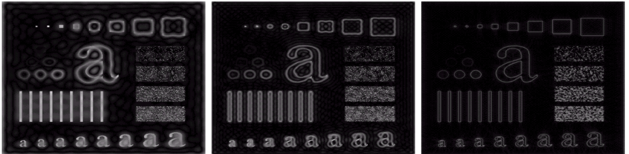
FIGURE 4.24 Results of ideal highpass filtering the image in Fig. 4.11(a) with D_0 = 15, 30, and 80, respectively. Problems with ringing are quite evident in (a) and (b).
