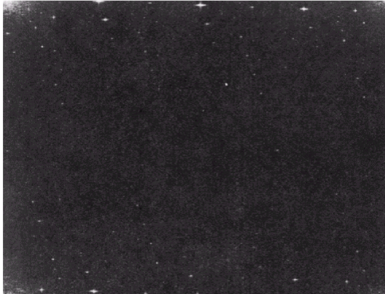
FIGURE 5.21 Fourier spectrum (without shifting) of the image shown in Fig. 5.20(a). (Courtesy of NASA.)
