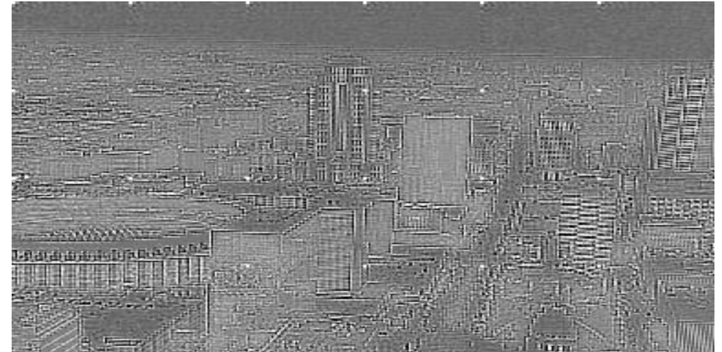
g) Error image comparing the original and (f), histogram stretched to show detail
