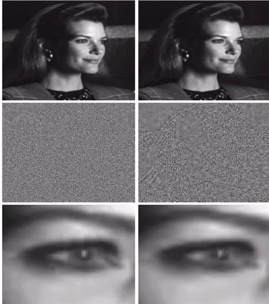
FIGURE 8.40 (a), (c), and (e) Wavelet coding results comparable to the transform-based results in Figs. 8.38(a), (c), and (e); (b), (d), and (f) similar results for Figs. 8.38(b), (d), and (f).
