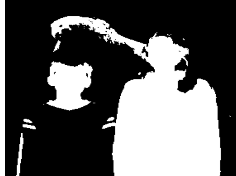
h) Image after reduction to 1 bit/pixel, 2 gray levels, compression ratio 44.46, with Gray code preprocessing 44.46
